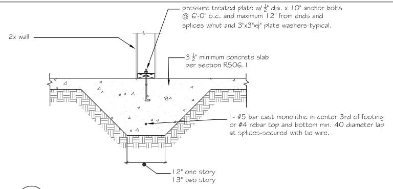
Interior thickened Slab at bearing walls or braced wall lines
